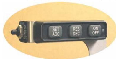
Safety is every bit as important as performance and QuadCruise has built-in failsafe features. Its minimum speed limit and neutral gear monitoring prevents a child jumping on and engaging the cruise control. It will also disengage at 15mph or above double the **SET** speed. The brake always disengages the control.
